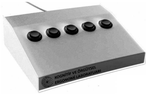
Figure 1. Response Box connected to the computer used in the experiment.
