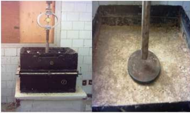
Figure7. Plate loading process on limestone subbase.
