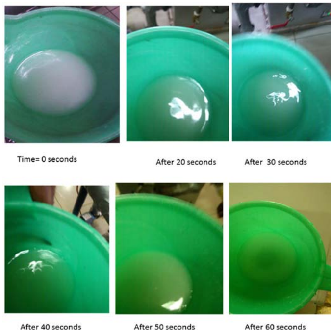
Figure 16. Hydrate dissociation when exposed to atmospheric conditions.
