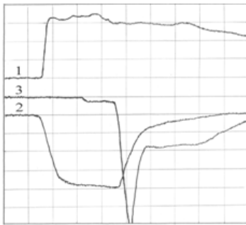
Fig. 16. Waveforms of the (1) incident wave voltage, (2) input voltage on the discharge tube, and (3) total discharge current (dimensional units). An arrow shows the instant of sliding discharge initiation. The time scale division is 10 ns. U_0 = U_{\text{inc}} = 60\ \text{kV} .
