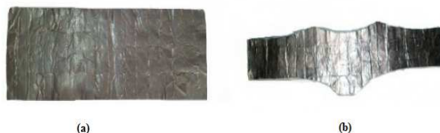
Figure 3. (a) Representation of lead plate without form of thyroid shield, and (b) in the final format.
