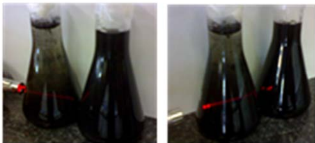
Fig. 2. Comparison of the stability of the SDS stabilized CNTs suspension (the right one) with the unstable CNTs suspension without SDS (the left one). The photos were taken after 3 days pH of both suspensions was kept 10.
