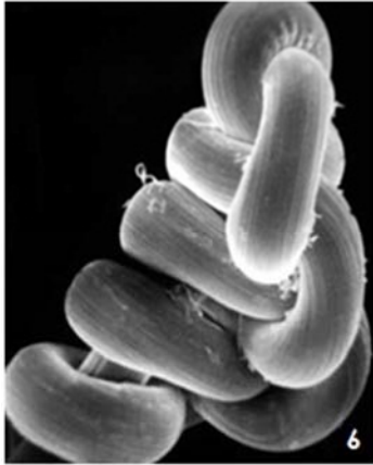
Figure 6. PREMILENE. Blue nonabsorbable polypropylene monofilament. (B/Braun). Knot x60.
