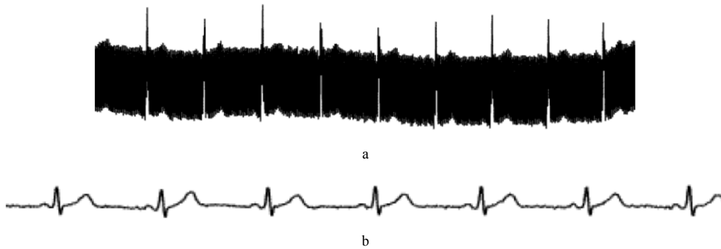
Figure 26. ECG signal from a 12 lead commercial ECG Machine (a) Before software filtering (b) After software filtering.
