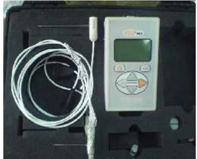
Figure 1. Thermal conductivity meter.
