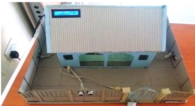
Figure 10. A model house with the microcontroller based home security alert system installed.
