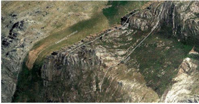
Figure 5. The sinistral, post-folding, ductile Villiersdorp fault in the cover sediments, resulted in north-north-east trending shearing on both the eastern and western limbs of the Villiersdorp syncline.
