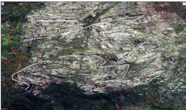
Figure 8. Doubly plunging folds, fracturing and shearing by tangential longitudinal strain in the more massively layered Skurweberg Formation, near Grabouw.
