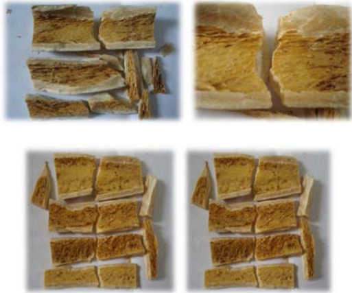
Fig. 10. Proximal and Distal regional (without crack) specimen subjected to impact load.
