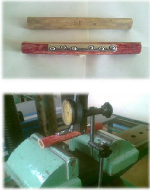
Fig. 4. a) Bending test specimens b) Test on UTM.
