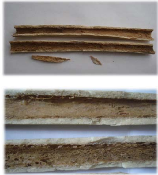
Fig. 15. With crack bending test specimen after test.
