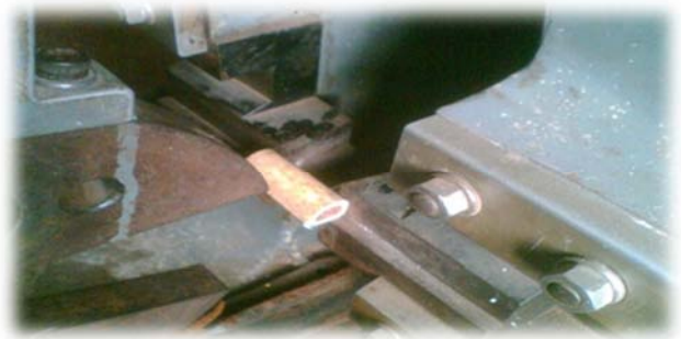
Fig. 3. a) Impact test specimen b) Testing on Impact testing machine.
