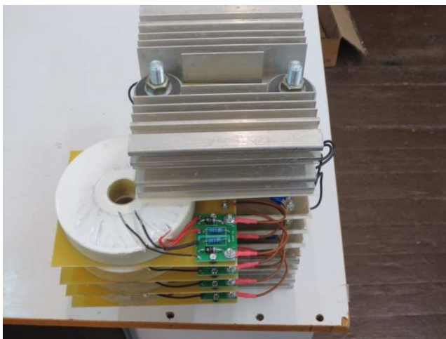
Figure 3. General view of a thyristor block with the current transformers and the elements thereto.
