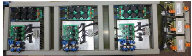
Figure 4. General view of the drivers for one thyristor group together with the power supplies.
