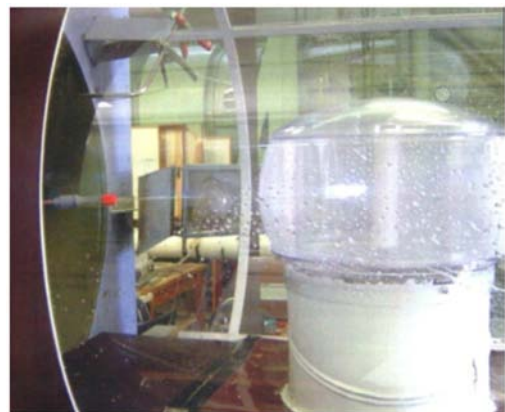
Figure 17. Plastic transparent ventilator with direct stream test.
