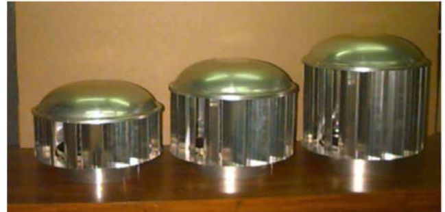
Figure 8. Turbo ventilator with blades heights 170 mm, 250 mm and 340 mm Hybrid.
