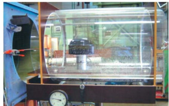
Figure 16. Aluminium ventilator with direct stream test.
