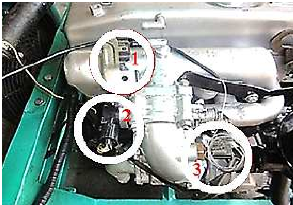
1 –MAF sensor; 2 – APP sensor; 3- THA sensor.
