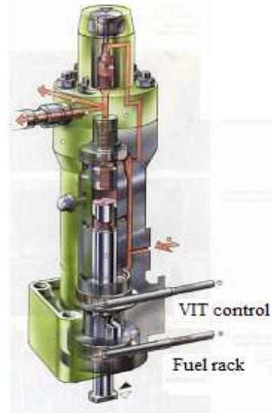
Figure 10. The Injection Timing Regulation VIT in MAN B&W engines
