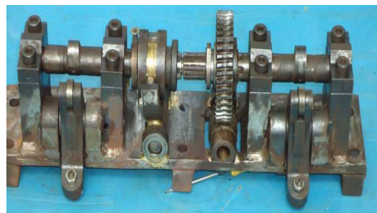
Figure 8. The mechanism for controlling cylinder deactivation.
