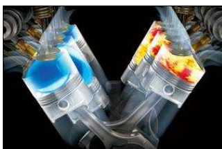
Figure 1. Cylinder deactivation for a 6 cylinder engine [1]
