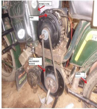
Fig. 15. (A, B, C & D) Hardware Implementation – SEFPHV.
