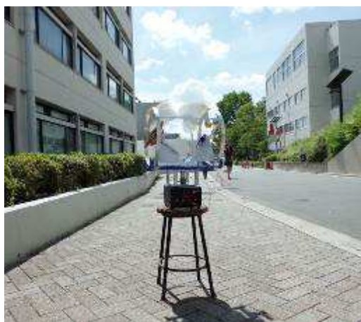
Fig. 1. Instrument for producing reduced metal nanoparticles from metal oxides using solar-pumped high-repetitive laser in action.
