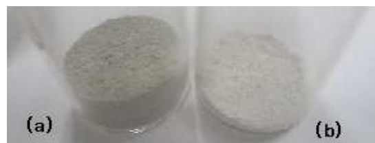
Fig. 4. (a) Mg(OH) 2 powder collected from Mg air cells and (b) after laser irradiation
