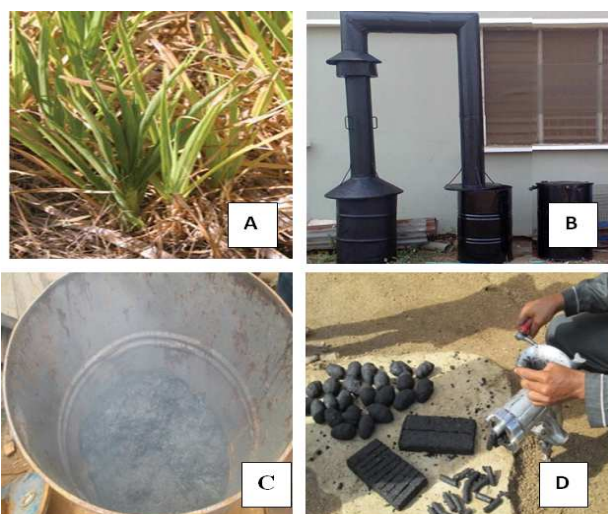
Figure 2. A: Elephant grass, B: Closed drum carboniser, C: Semi-finished product and D: Finished product (pellets)
