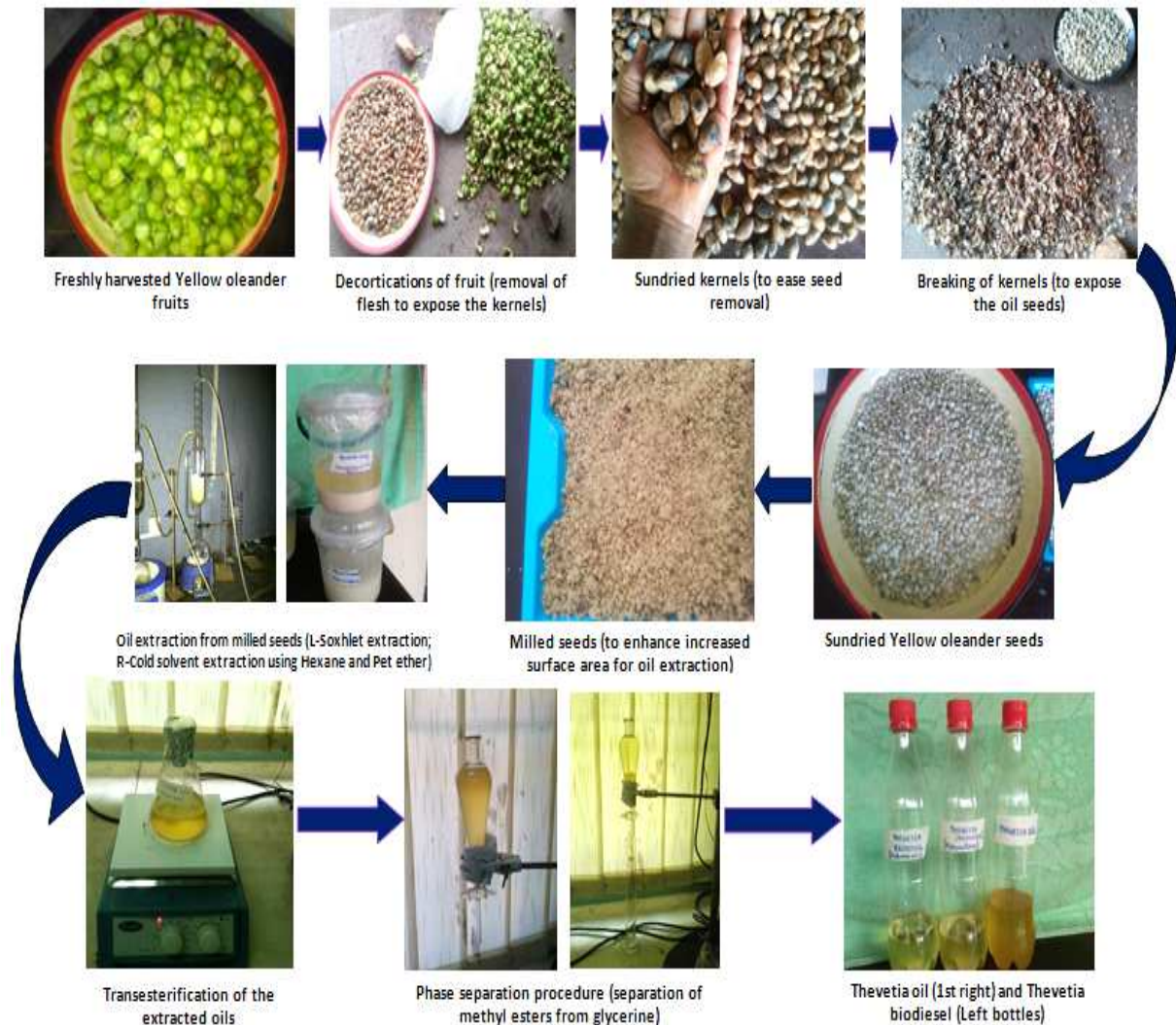
Figure 2. Highlights of the major steps involved in the production of biodiesel from Yellow oleander fruits.
