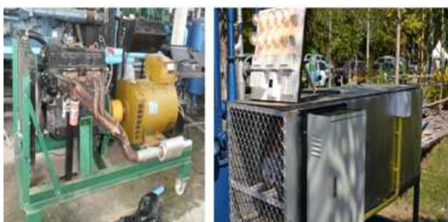
Figure 5. producer gas engine and load (heater).
