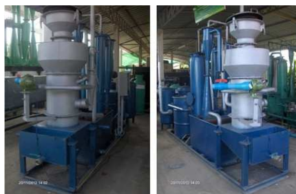
Figure 2. Producer gas Down Draft type.
