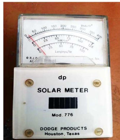
Fig 4. Solar power meter
