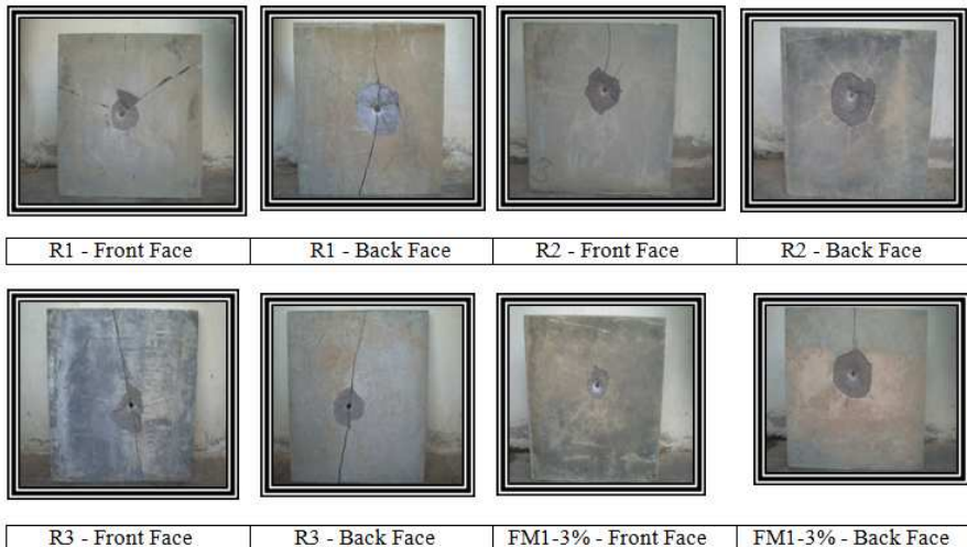
Fig. 18. The Mode of Failure of Slabs under High Velocity Impact
