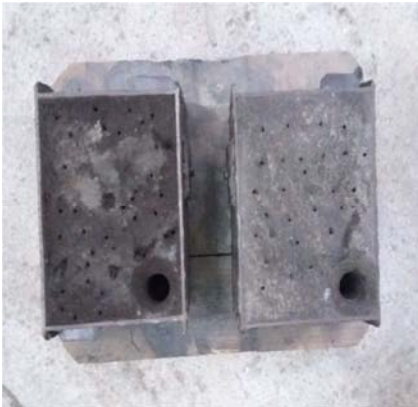
Figure 6. Mold for casting.
