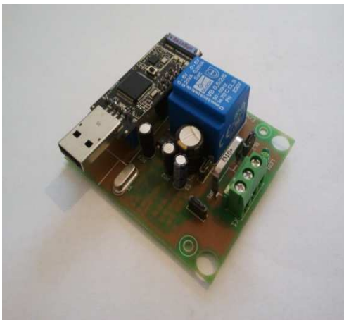
Figure 5. Electric sensor used as a relay node.
