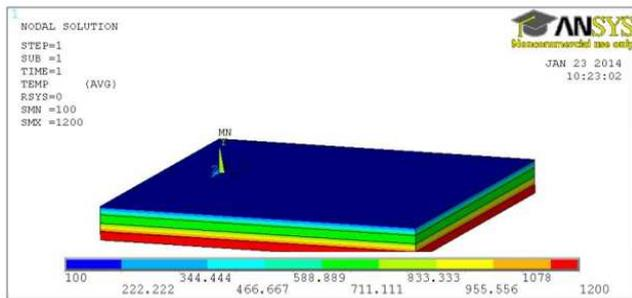
Figure 3. Heat distributions through the four-layer structure.
