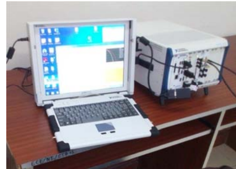
Figure 3. NI PXIe VST based Set-up for LTE.
