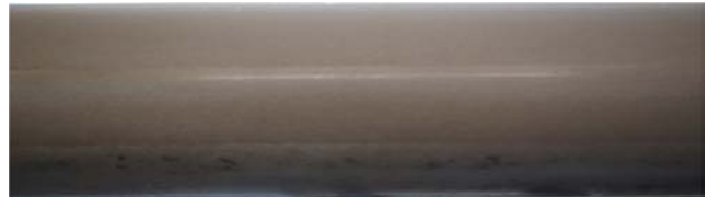
Figure 4. Stratified flow when the velocity of main flow is low.
