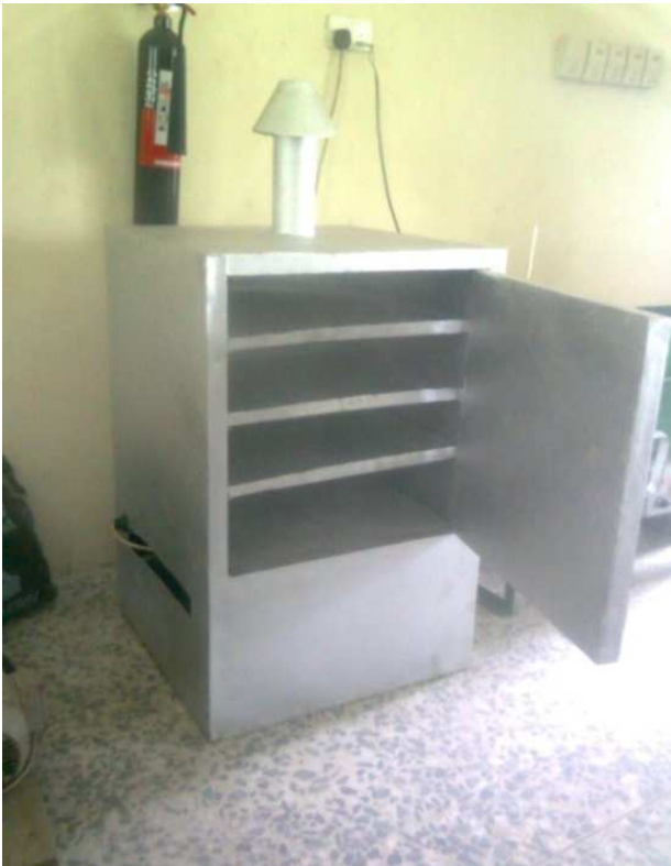
Figure 1. Fabricated cabinet tray dryer.
