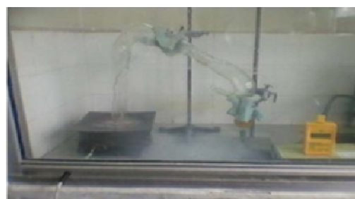
Figure 1. Spray pyrolysis experimental set up.
