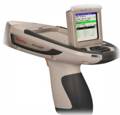
Figure 3. X-ray fluorescence spectrometer, the Niton XLT900s.
