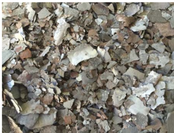
Figure 1. Appearance of lump scale from steel feed after reheating furnace.
