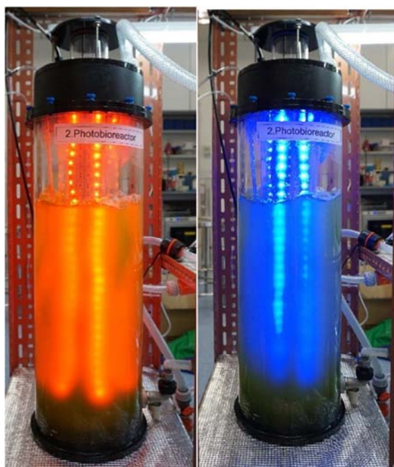
Figure 2. Photograph diagrams of the internally-illuminated photobioreactor under red and blue illuminations.
