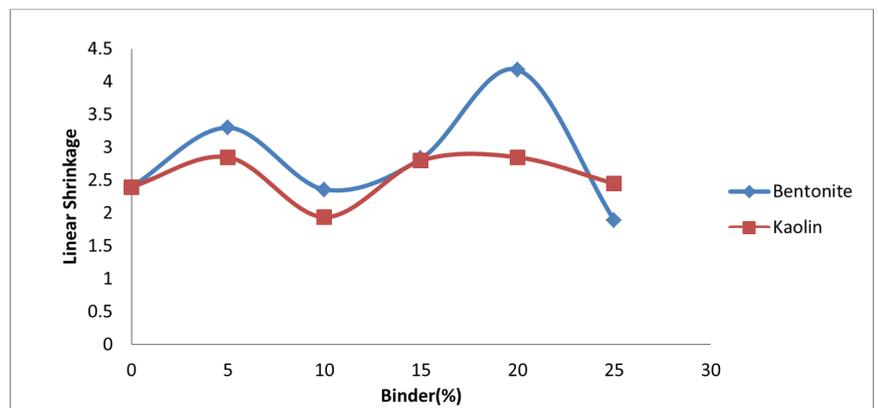
Figure 8. Linear Shrinkage of Ile-Ife Anthill Clay.
