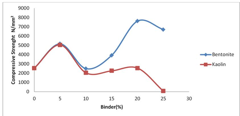
Figure 7. Compressive Strength of Akure Anthill Clay.
