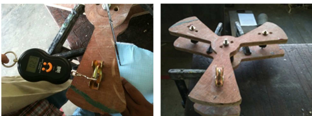
Figure 5. Diamond connection model (left) Test (right).
