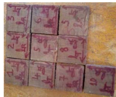
Figure 4. WW specimens of 50 \times 50 \times 10 \text{ mm}^3 .
