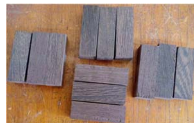
Figure 3. WW specimens of 60 \times 20 \times 20 \text{ mm}^3 .
