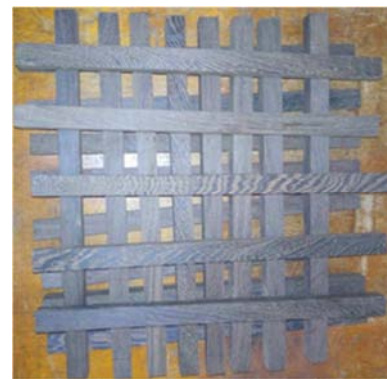
Figure 2. WW specimens of 360 \times 20 \times 20 \text{ mm}^3 .
