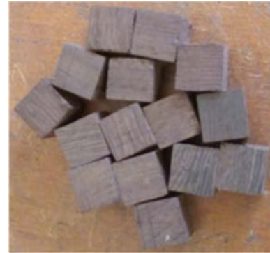
Figure 1. WW specimens of 20 \times 20 \times 20 \text{ mm}^3 .
