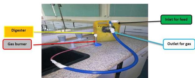
Figure 2. Pilot scale digester of 10 L capacity.
