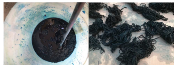
Figure 18. Leather strips soaked in dye and placed under a shade to dry gradually.
