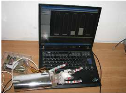
Fig. 2a. First anthropomorphic hand prototype - mechanical structure
