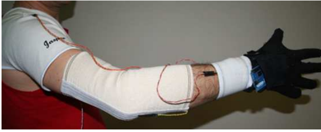
Fig. 9. Joint sensors
