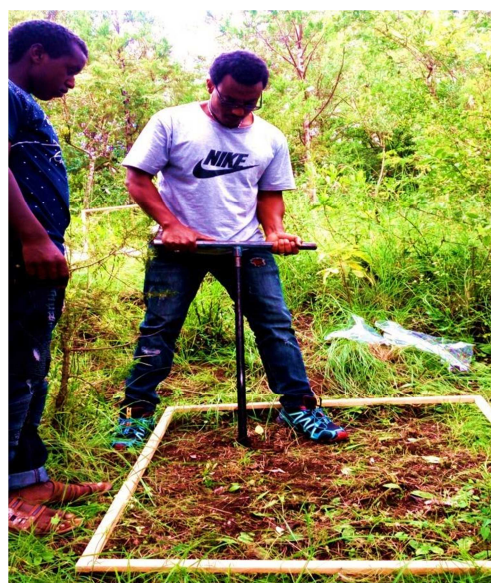
Figure A3. Soil sample collection.
