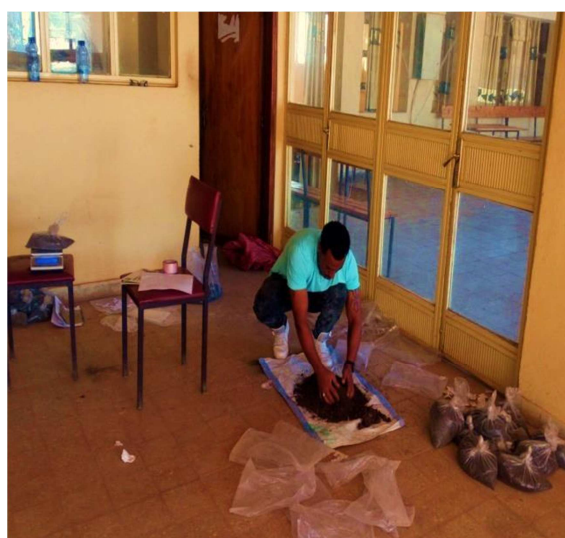
Figure A4. Disturbing composite soil samples.
