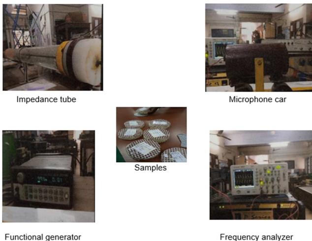
Figure 6. Standing wave apparatus (Source: Indian Institute of Technology Chennai).
