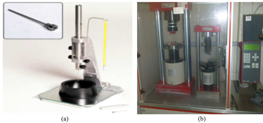
Figure 2. (a) Vicat apparatus and (b) Toni Technik compression machine.
