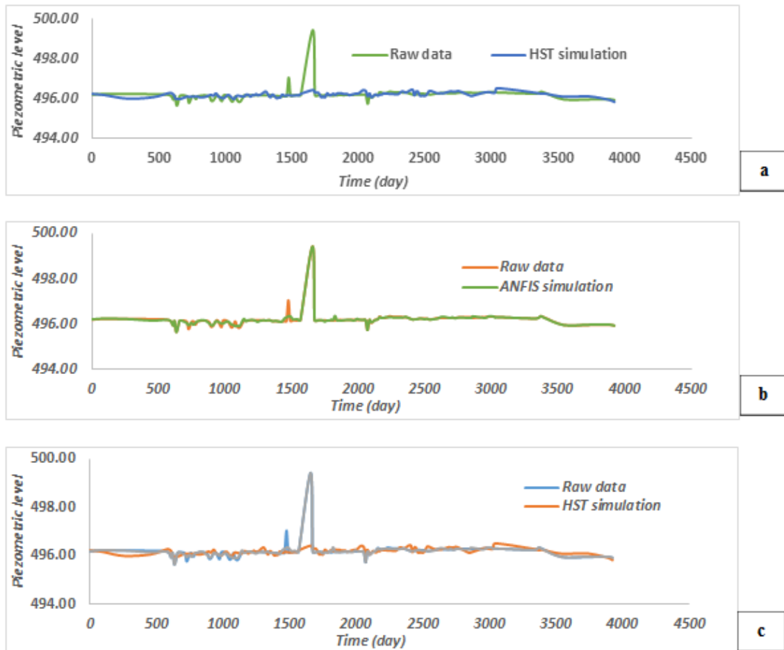
Figure 16. Comparison of the different behavior models of the I3 piezometer.
