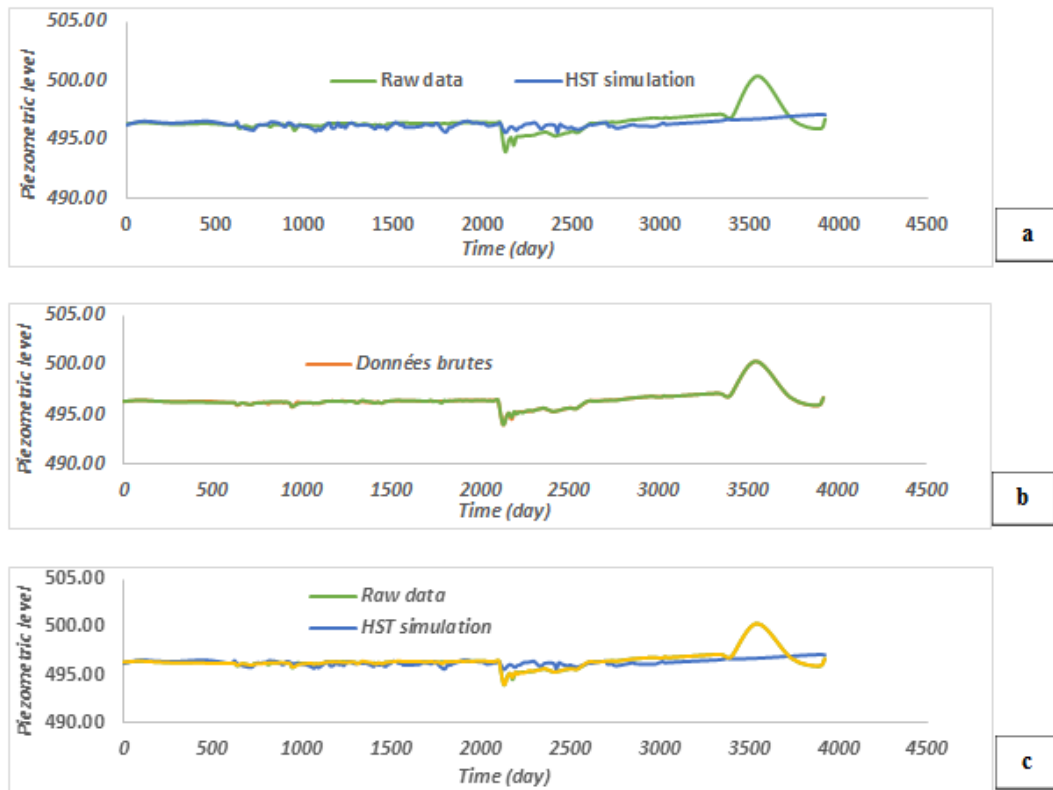
Figure 12. Comparison of the different behavior models of the I2 piezometer.
