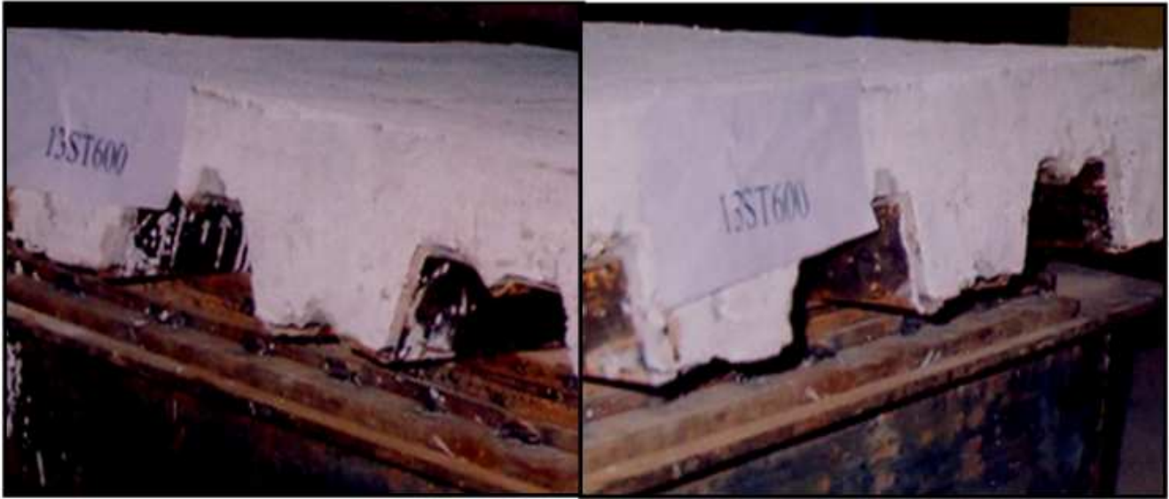
Figure 8. Typical end slips for L_s = 600 mm from left & right side of specimen.
