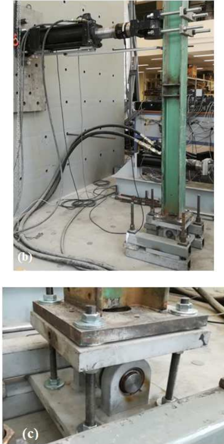
Figure 6. (a), (b) Test setup, (c) clevis connection.
