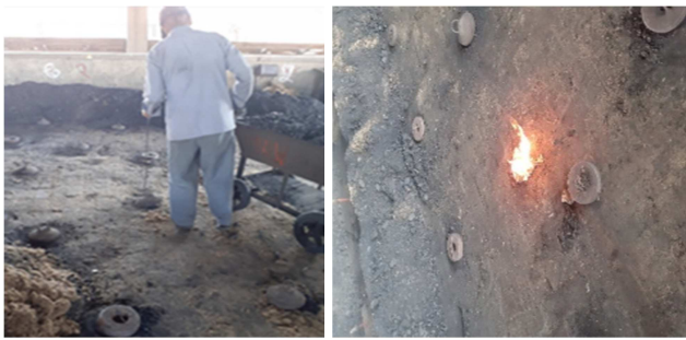
Figure 6. (a): Setting for burning fuel, b) brick burning.
