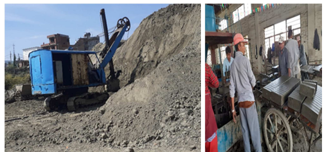
Figure 2. (a): Taking Brick clay from storage place near the factory; (b) Green bricks ready to firing.
