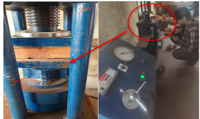
Figure 9. Compressive Strength Test of Brick Samples.
