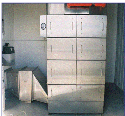
Fig. 9. Air purification unit scaled up for large volume air intake.
