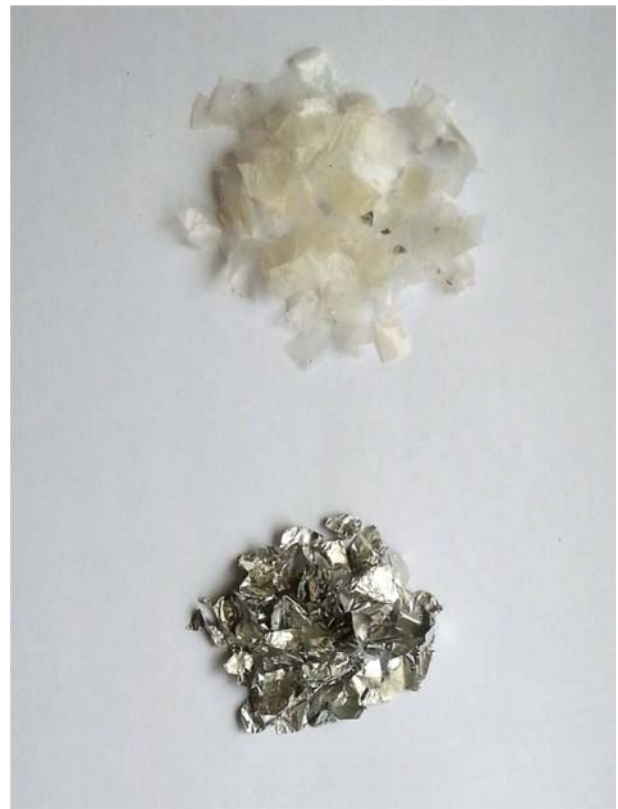
Figure 6. Products obtained from PE-Al laminate by delamination with 20% formic acid at 40°C: LDPE flakes containing some Al contamination (top); aluminium based fraction (bottom).
