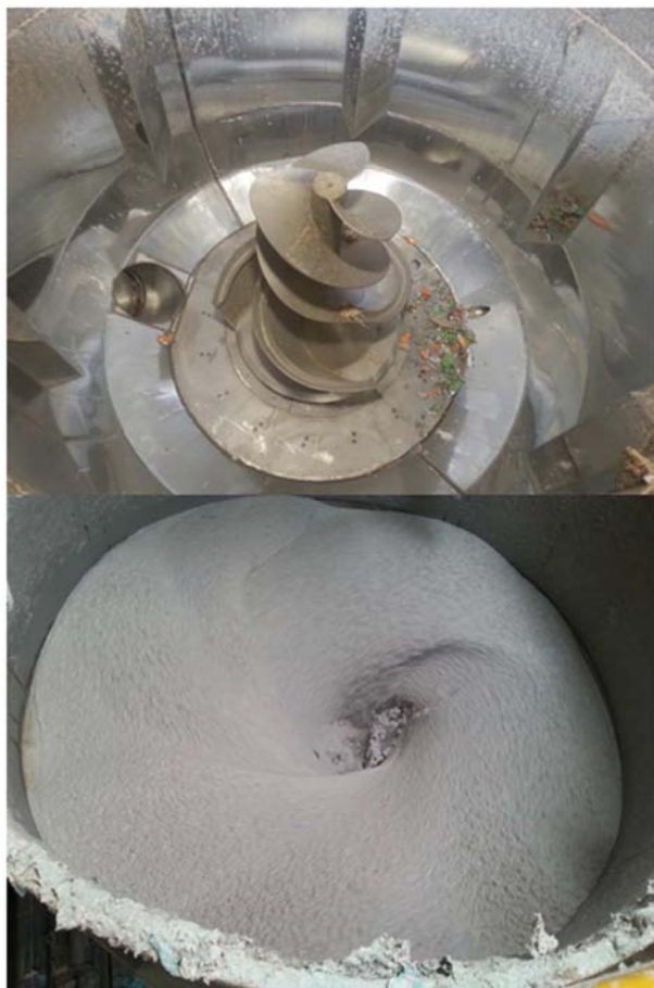
Figure 3. Vertical type hydrolpulper: empty (top); during UTPC processing (bottom).
