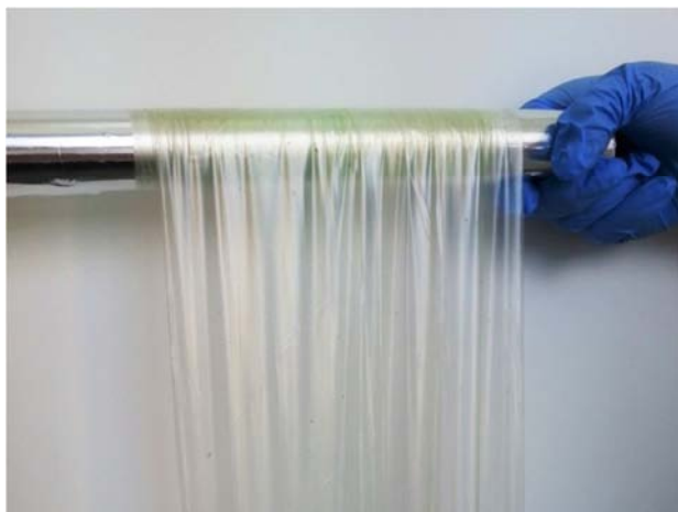
Figure 8. LDPE derived from PE-Al by solvent extraction could be successfully used in blown film extrusion process.
