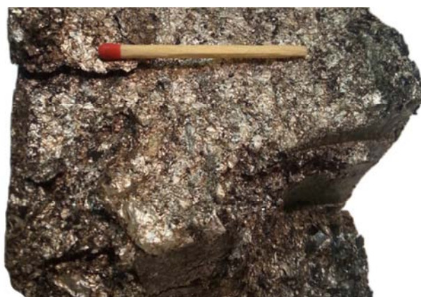
Figure 4. Solid product of pyrolysis process. Composition: 42,9% C; 36,9% Al total ; 17,7% Al met .
