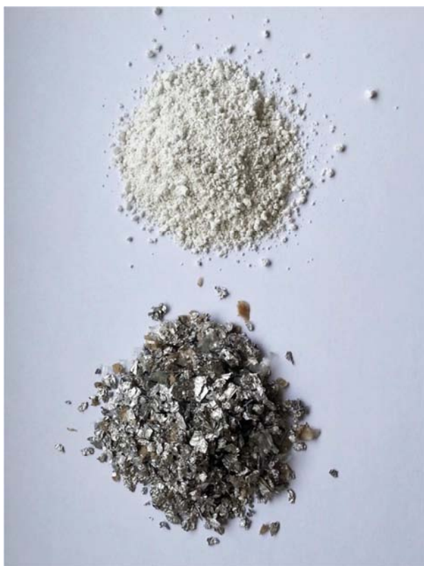
Figure 7. End-products obtained from PE-Al laminate by solvent extraction process: nearly white LDPE powder (top); aluminium based fraction: 59,9% Al_{met} , 0,9% Al_{ox} , 35,2% organic impurities such as paper, PET, residual LDPE etc. (bottom).
