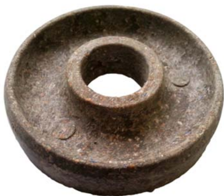
Figure 1. Core plug used to protect paper mother rolls during transportation.
