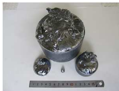
Figure 12. Many kinds of shapes “Liquinert” poly-Si.
